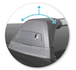
CAUTION: Recheck all fasteners immediately after a load is applied to the crossbars. Regularly check screws are tight.
