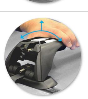
• Check crossbar is securely attached to the vehicle.
