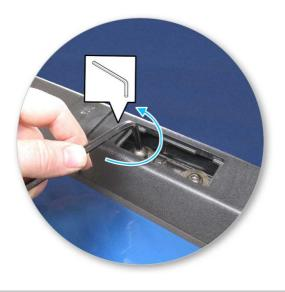
Remove M8 mounting bolt from fixed-point using 4mm hex key, as shown.
