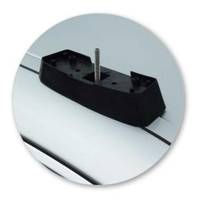
It is important to put the pads in the correct position on the vehicle.
