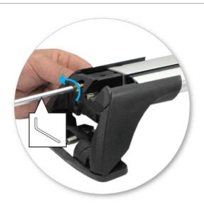
Use hex screwdriver to reverse adjusting screw 10 turns.
