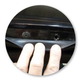
Pull back rubber seal to expose fixed points on vehicle body.
