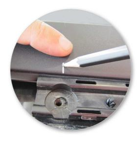
Mark reference point with a pen onto removed section of ditch mould.
