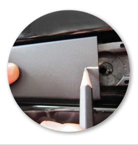
Mark reference point with a pen onto removed section of ditch mould.
