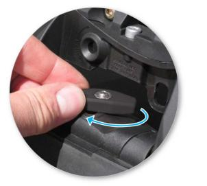
• Tighten the plastic knob. The side with the nut showing should be facing up.
