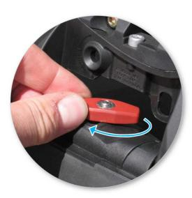
• Tighten the red plastic knob. The side with the nut showing should be facing up.
