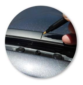
Mark a reference point for the front and rear mounting points with a pen as shown.
