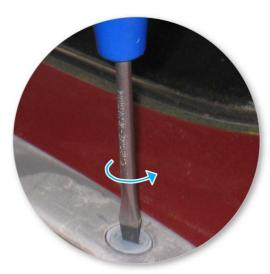
• Remove plastic plugs from fixed points in the roof with a flat-head screw driver.
