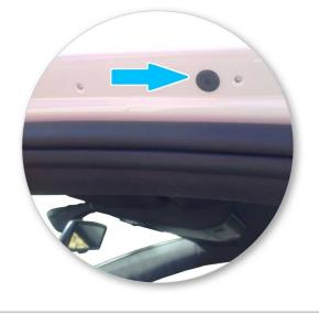
Locate vehicle's fixed points for the front bar.
