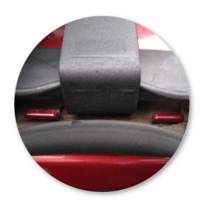
Slide clamp into the fixed point ensuring that it is fully engaged.
