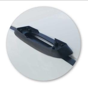
Put rubber pad (supplied with crossbar) on the vehicle.
