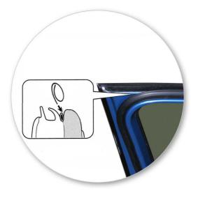
• Ensure door seal positioned as shown.
